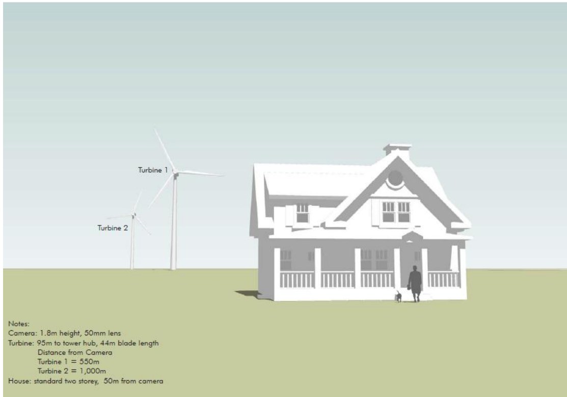
Visual Aid 1: Wind Turbine Scale Schematic
